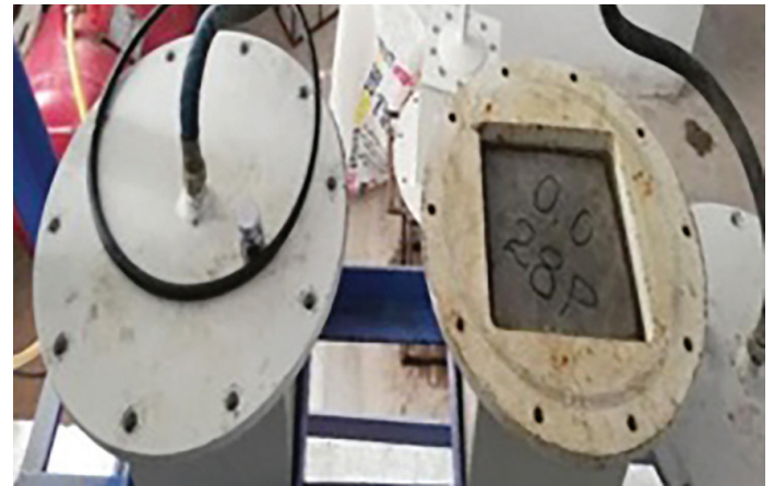
Figure 3: Cube inserting position in a cell
