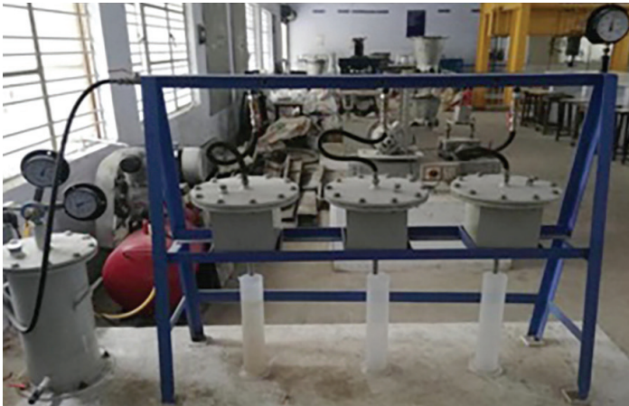
Figure 2: Water permeability test set-up
