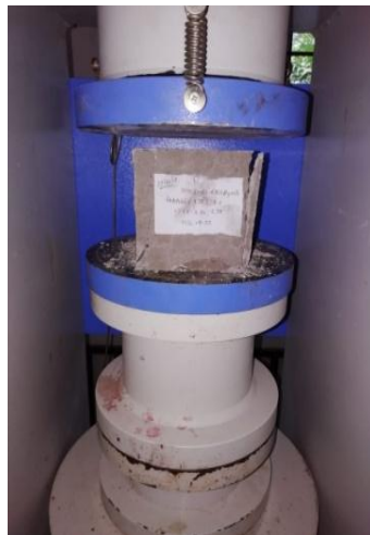
Fig 4.1-load acting on cube
